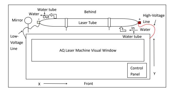
After connecting the water pipe of laser tube, remember to rotate the laser pipe to adjust the water inlet to the lower part, the water outlet to the upper part, and then fix the bracket.
